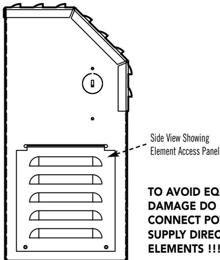
**TO AVOID EQUIPMENT DAMAGE DO NOT CONNECT POWER SUPPLY DIRECTLY TO ELEMENTS !!!**
