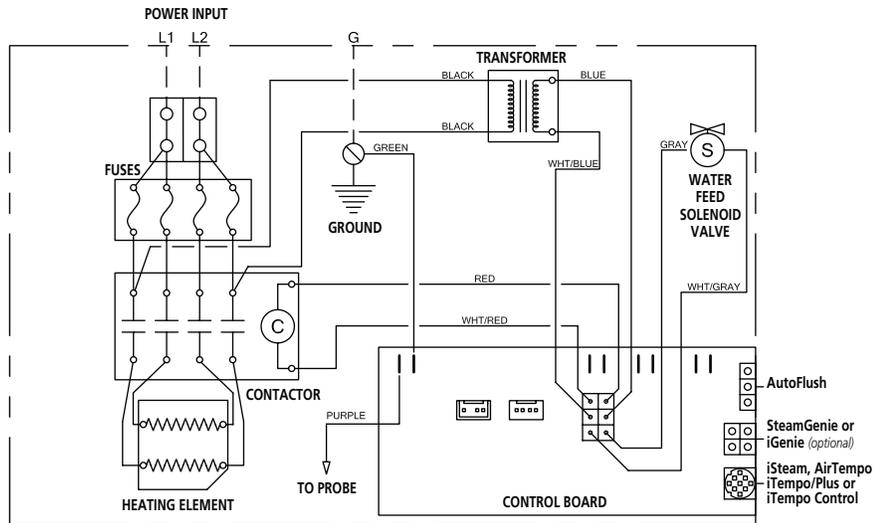
**THREE PHASE 208/240 VOLT WIRING DIAGRAM**
