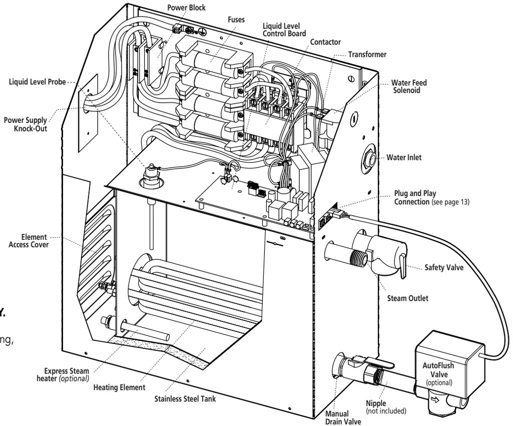
**NOTE:** Super 1E 240/1 models are not supplied with internal fusing.
